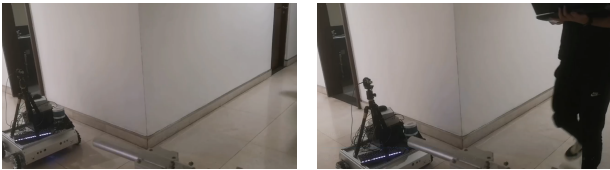
(a) The vehicle moves when no approaching object is found (b) The vehicle brakes when the approaching object is found
